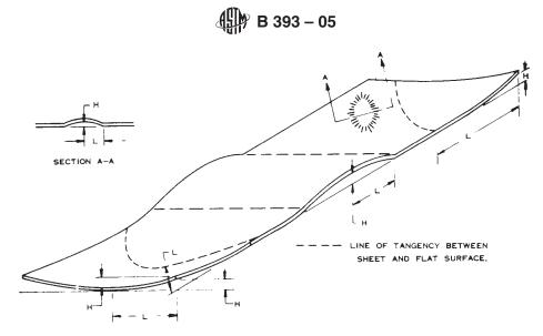
H = maximum distance between flat surface and lower surface of sheet. L = minimum distance between highest point on sheet and point of contact with flat surface. Flatness, percent = (H/L) x 100
